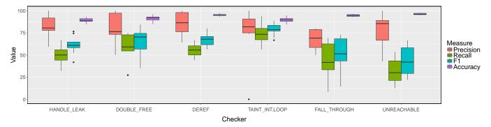
Fig. 10: Boxplots of precision, recall, F1, and accuracy metric from ten-fold cross validation of classifier training for each studied static analysis checkers. Median precision is over 75% for five out of six checkers, while median recall is over 50% for four out of six studied checkers.
