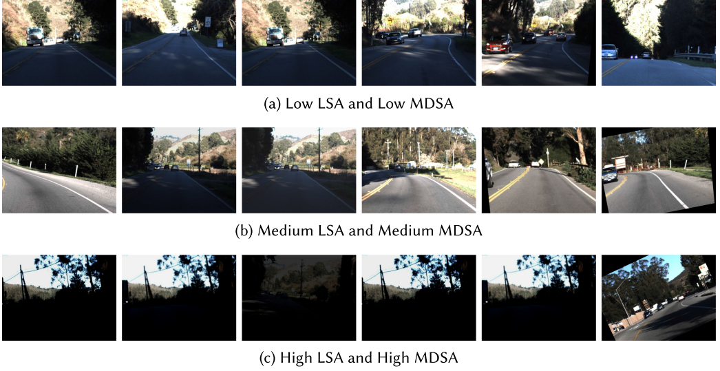
Fig. 3. Synthetic images for Chauffeur model generated by DeepTest. The three images on the left are picked based on LSA and three images on the right are picked based on MDSA. Images with higher LSA or MDSA values tend to be harder to recognize and interpret visually.
